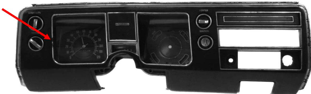
2. Remove the five screws holding the gauge cluster to the dash panel. Save this hardware as it will be reused.
