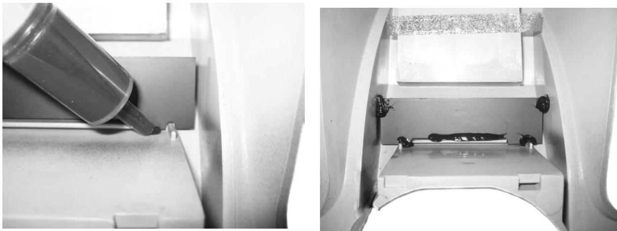
6. Install the HDX system into the stock lens spacer by securing the system to the spacer by reusing the seven screws removed in step 3.
