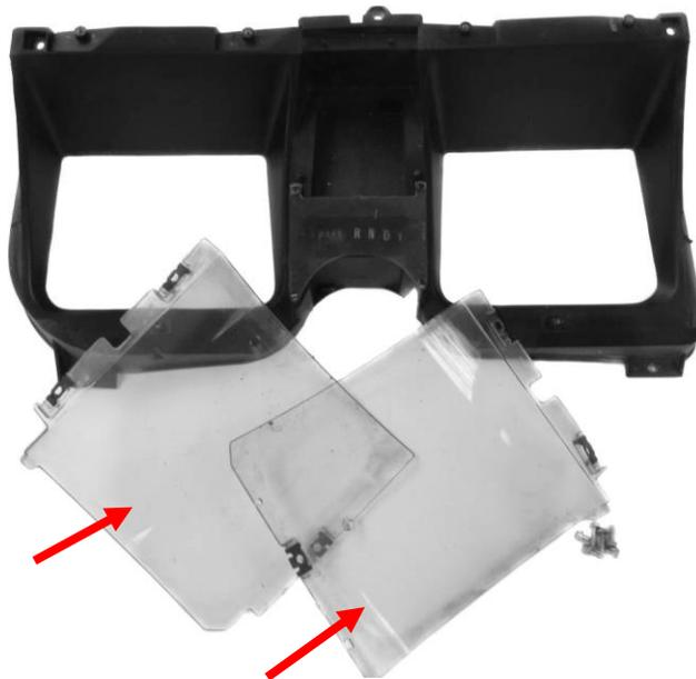
5. This step is optional for automatic transmission bezels only. If you purchased a separate GSS universal gear kit from Dakota Digital, the gear position can be displayed in the HDX message centers; therefore the stock gear position indicator can be removed.
