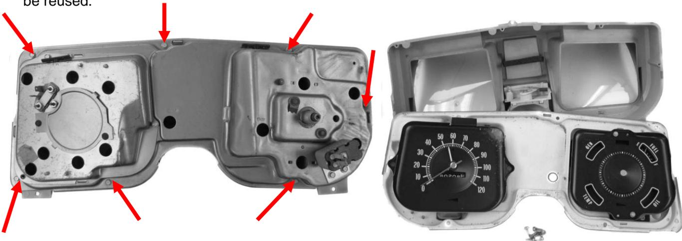
4. Remove the stock lenses from the lens spacer by removing three screws from the front of each lens. The stock lenses are removed since the new HDX kit features hard coated clear lenses.
