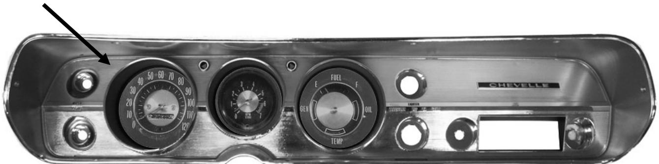
2. Remove the stock gauge, and lens from the bezel. The only item to be reused is the original front bezel.
