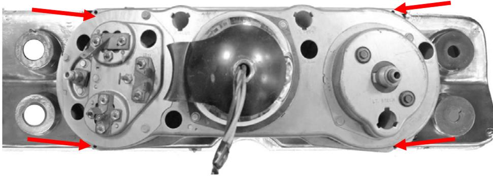
3. Secure the HDX system to the bare bezel using the supplied screws.
