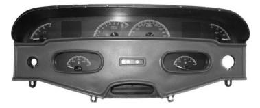
7. Removing the stock gauge eliminates the illumination for the gear indicator during headlight. The supplied gear indicator block off lens can be used if so desired.
