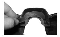
10. Reassemble lower dash bezel when the silicone has cured.
