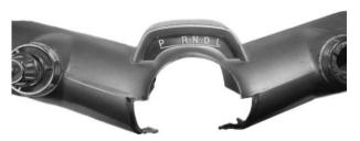
8. With the lower dash bezel already out, remove the two mounting screws to remove the indicator plate and lens.
