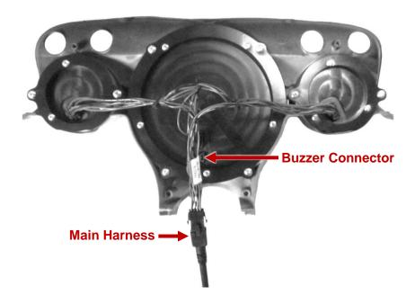
6. Re-install the cluster into the vehicle using the retained factory hardware. Refer to the main HDX manual for wiring instructions to complete the installation.
