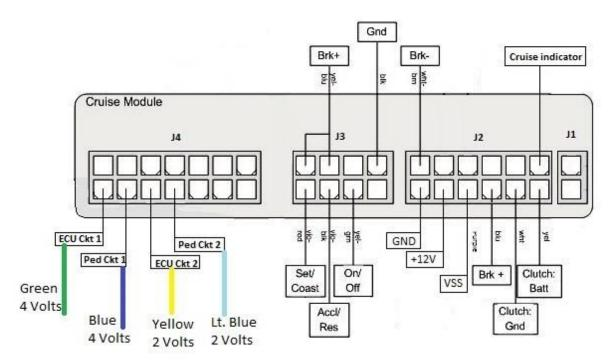
Note: Voltages are with the accelerator pedal fully pressed to the floor. Ensure the key is in the 'on' position and the engine is NOT running.
