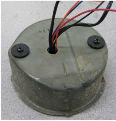
5. Slide the gauge into the can making sure not to pinch the wires when it is fully installed. Through the original light bulb holes install the screws and large plastic washers. Snug but don't fully tighten the screws so alignment can be adjusted.
