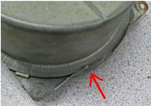
2. Bend open two or three crimps holding the two can halves together and separate them.
