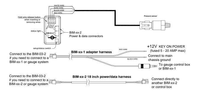
This Bus Interface Module connects to a solid state pressure sensor. There are two power & data interface (I/O) ports on the module. Either one can be connected to the gauge system or to another module, allowing several units to be daisy chained together. Do not connect the I/O port to anything other than a Dakota Digital gauge or BIM. Do not mount the module in the engine compartment; it should be mounted in interior of the vehicle.
